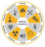
Example of Energy Wheel Developed by Quanta Services https://www.quantaservices.com/safety/the-capacity-model
